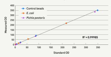
03 **Linearity of Optical Density on Cedex Bio HT Analyzer.** Measurements of control beads, *E. coli*, and *Pichia postoris*. (Roche Diagnostics evaluation data)
