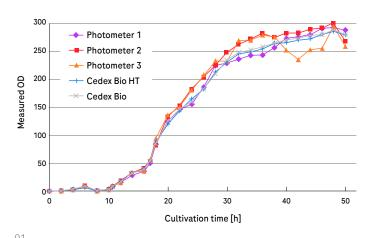
Method comparison: Optical Density of *E. coli* culture. The Cedex OD measurements show tight inter-instrument alignment and correlate well with the determination on three manual photometers. (Reference: Genentech evaluation data)
